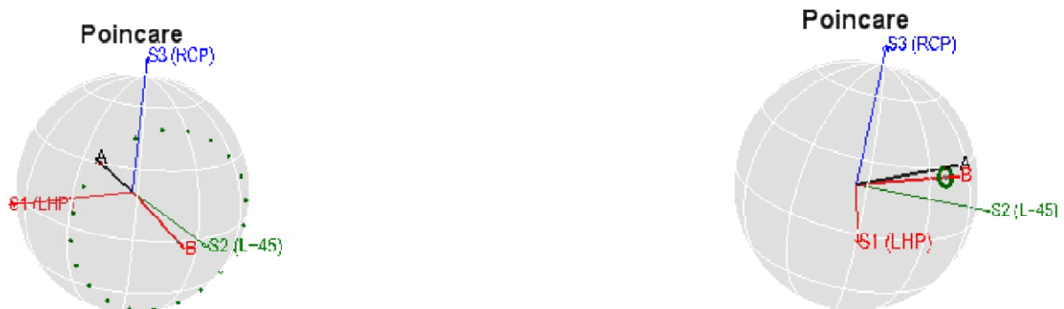
Figure 1. Evolution of the probe SOP along the transmission line (green circles) for different launch SOPs of probe (A) and pump (B).
