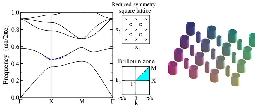
**Fig. 9.** Band-gap structure of the reduced-symmetry photonic crystal with  $r_0 = 0.1a$ ,  $r_d = 0.05a$ , and  $\varepsilon = 11.4$  for both types of rods. Full lines are calculated by the MIT Photonic-Bands program [31] whereas dashed line is found from the effective discrete model. The top center inset shows a cross-sectional view of the 2D photonic crystal depicted in the right inset. The bottom center inset shows the corresponding Brillouin zone.
